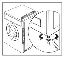
The machine must not be installed in rooms where the temperature can drop below 0°C. The water inlet hose and the drain hose must not be kinked.
